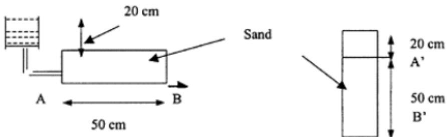
Note, the end of each column is free draining, i.e., pressure is atmospheric
