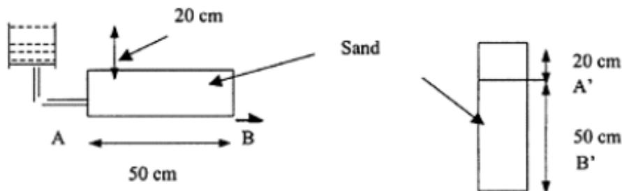
Assuming a reference point at the bottom of the vertical soil column, the pressure and gravitational head for the vertical flow are 20 cm and 50 cm, respectively, at point A'. At point B' both are zeros. The Darcy's flux through this soil column
